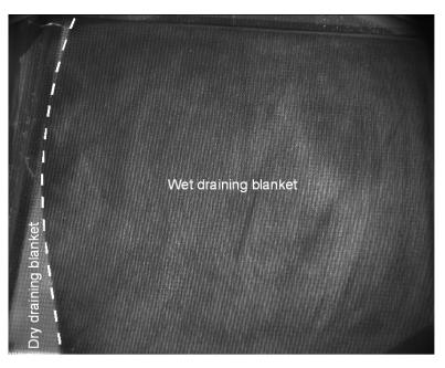
Fig.5 Resin propagation in the draining fabric.
