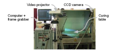
Fig.3 Experimental testing device
