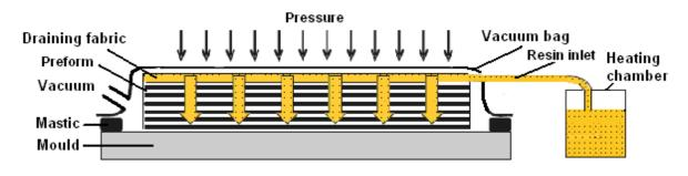
Fig. 1 Principle of LRI processes [1]
